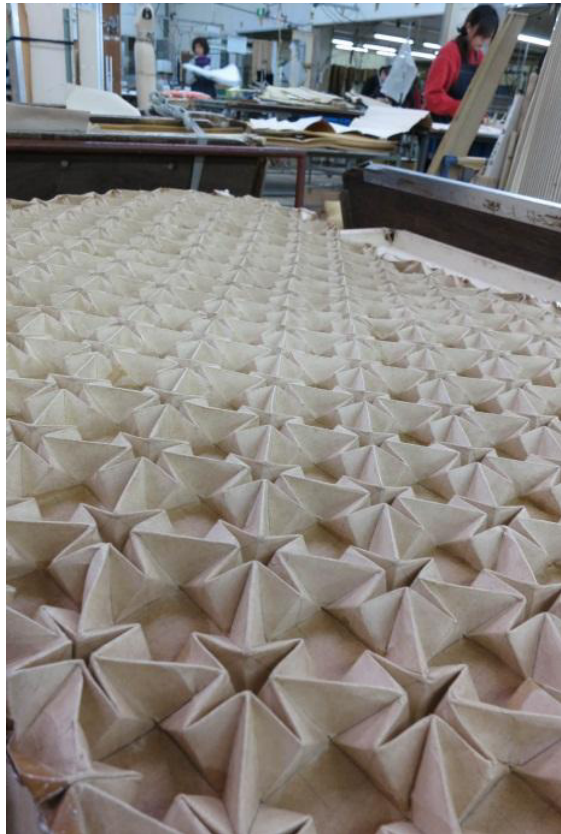
Images 17, 18, 19 and 20. Clockwise from upper left: close-up of polyester folds; hand-folding; resulting paper molds; heat-pressing installation
